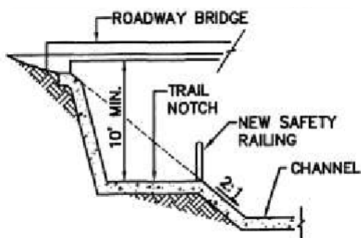
Figure 11: Trail Underpass Notched Into Side of Channel
