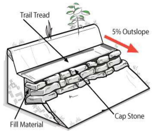
Figure 6: Typical MPOS Design for Natural Retaining Walls
