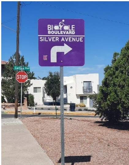
Figure 3: Wayfinding Sign with Route Name Identification and Advance Turn Notice
